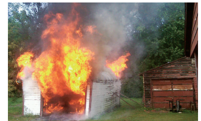
Despite the intense heat and flame, all we observed was a little blistering on the old siding.
